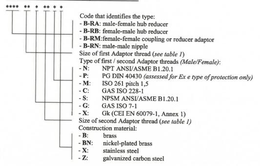
The Adaptors type B-RM and B-RN have both NPT threads or both Metric threads or coupling NPT-Metric threads.
